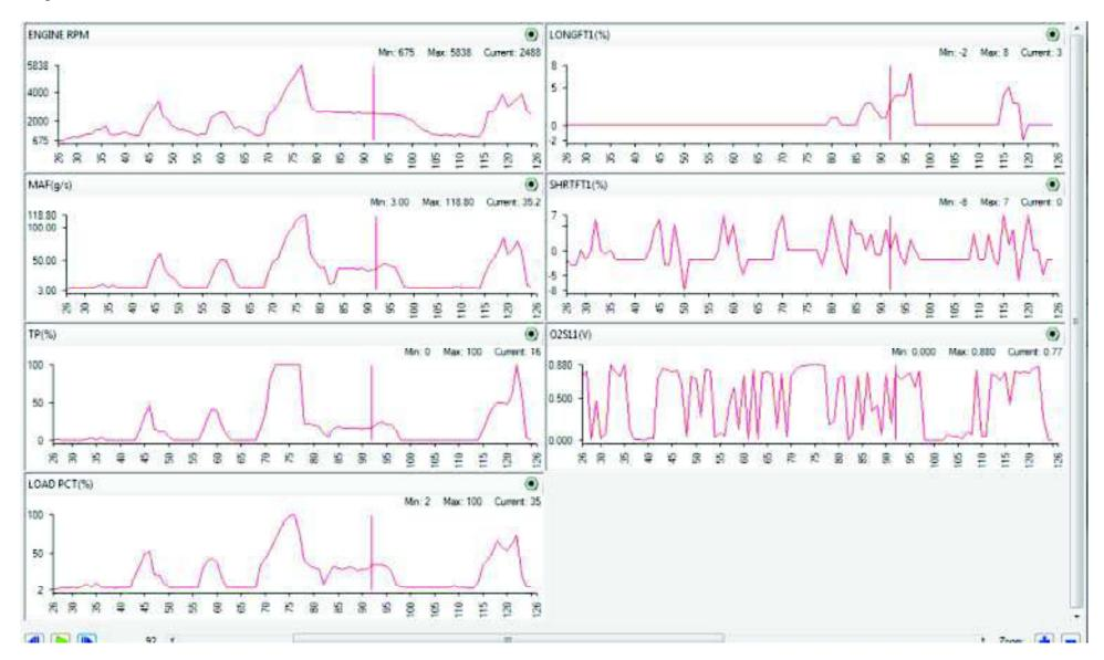
Pay close attention to the way the fuel trim graphs trend from low to high. I call this trend "digital," because the movement from -29 percent to zero percent is almost vertical, and the short term is also following the throttle movement. Here is a case where the information found in the trend of the fuel trims is of great value.
