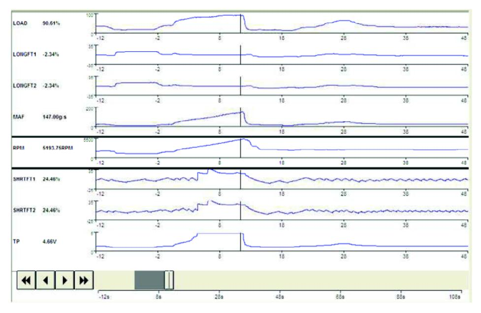
The MAF engine measures the actual air that is flowing through the MAF sensor. Things like restricted air intakes, restricted exhaust and EGR flow will not affect the air/fuel ratio. Take a look at the scan data where I have opened and closed the EGR valve. Notice that there is no fuel trim shift when the EGR is flowing. The EGR acts as cylinder filler and the air that is entering the engine has the proper amount of fuel injected to keep the
