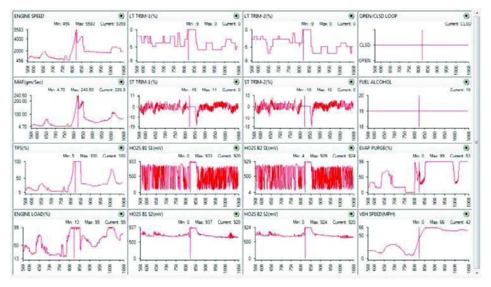
Many times we have heard that oxygen sensors sense oxygen. Well in a way they do, but in a way they don't. Oxygen sensors will react to oxygen, but they also react to the other gasses that are in the exhaust system. Things like hydrogen and carbon will cause the oxygen sensor to react, and unburned hydrocarbon (unburned gasoline) will cause the oxygen sensor to react differently. Knowing this will allow you to use the fuel trim information to analyze things like misfires or dribbling injectors.
