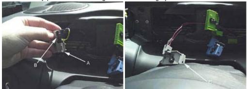
2. Connect the Mode Up wire by putting a Molex connecter in Slot 22 (2001-) or Slot 21 (1997-2000).
