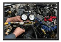
Step 3 - Record leakage percentage for the cylinder. Remove the oil dipstick, radiator cap, and oil filler cap. Open the throttle body or remove the air cleaner. Listen and watch. Wherever air is escaping will indicate where the problem is. Disconnect the gauge and move onto the next cylinder.
