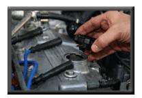
**Step 2 -** Figure out which spark plug adapter works best and connect the gauge into the hole. Put the vehicle in gear and set the parking brake to prevent the engine from turning when air is compressed into the cylinder. Start with the regulator turned counterclockwise to zero the incoming pressure. Connect compressed air. Turn the regulator clockwise to pressurize air into the cylinder.
